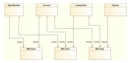
Fig. 2: SpecIF system model derived from the SpecIF meta-model with interrelated *ObjectTypes* used for diagrams and model-elements
