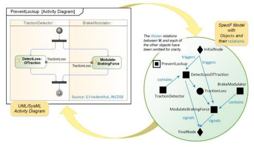
Fig. 4: An example activity diagram in SysML notation (left) and the corresponding SpecIF model (right).
