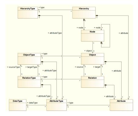
Fig. 1: The SpecIF meta-model derived from the OMG meta-object facility (MOF).
